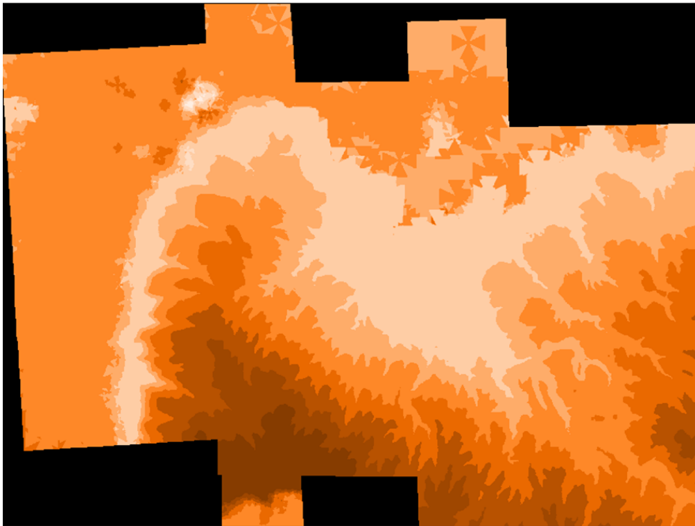
Figure 14: DEM (5x5 cm grid) generated at ENEA, from SHOA aerial photos (1:15000).
