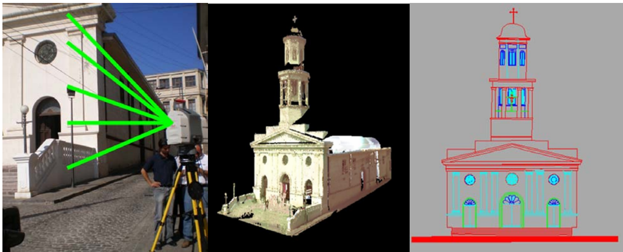
Figure 17. 3D laser scanner process.
