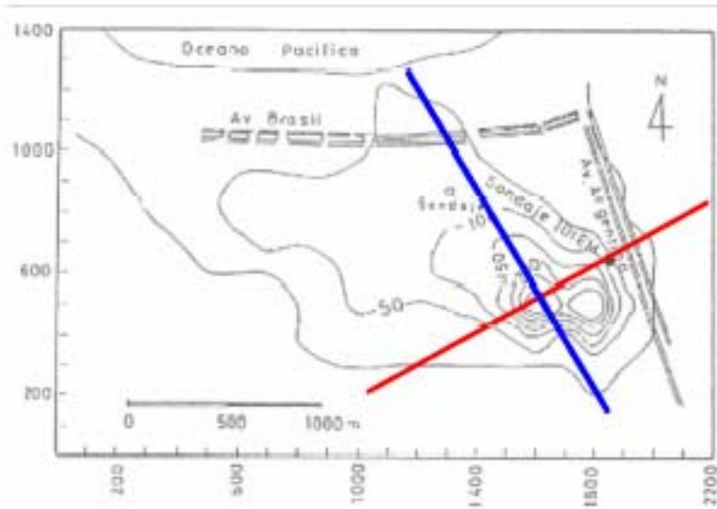
Figure 33: Bedrock model (depth) at El Almendral (Verdugo, 1995; Saragoni 2006) and the position of the two profiles.
