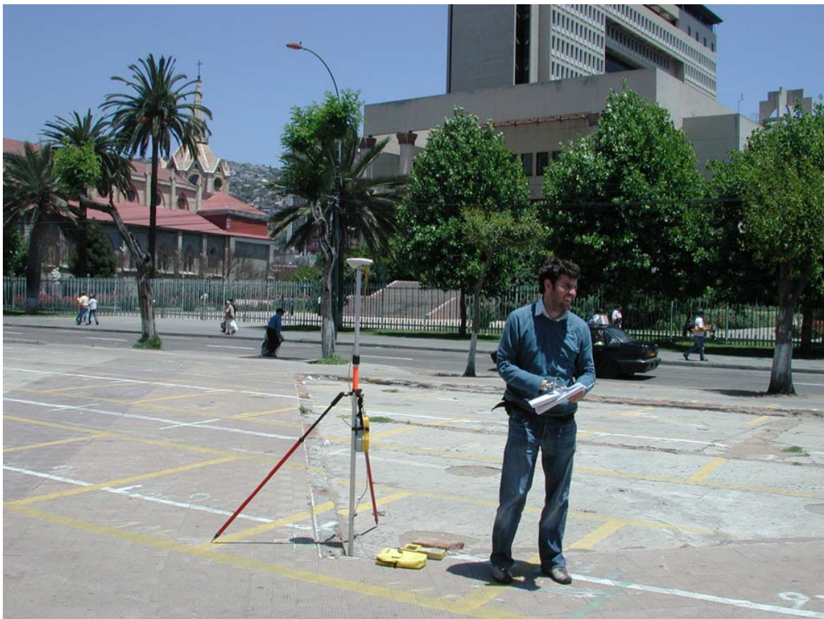
Figure 12: DGPS Rover on site ARGENTINA 2.
