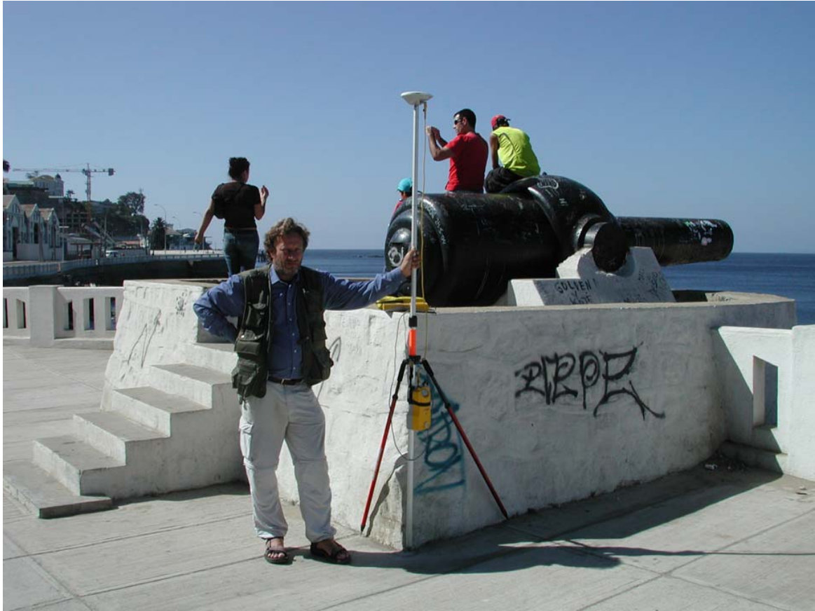
Figure 13: DGPS Rover on site ARMA.
