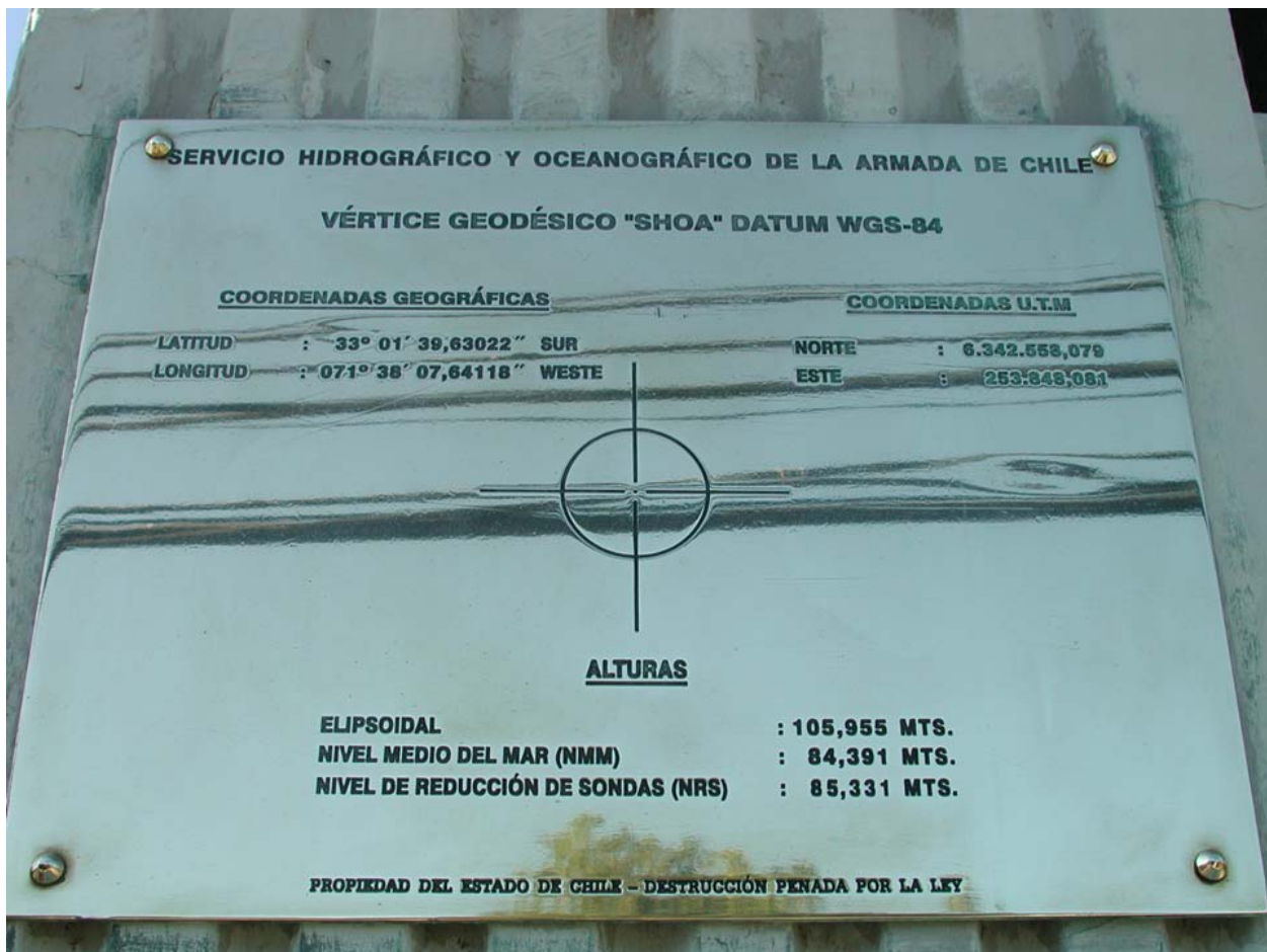
Figure 2: SHOA trigonometric vertex with Geographic and UTM coordinates.
