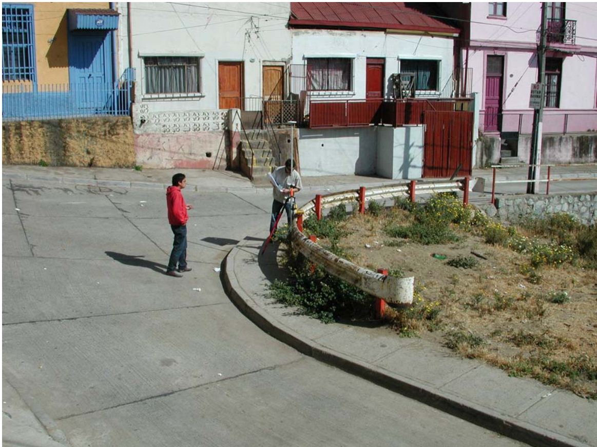
Figure 14: DGPS Rover on site AUGUSTIN.
