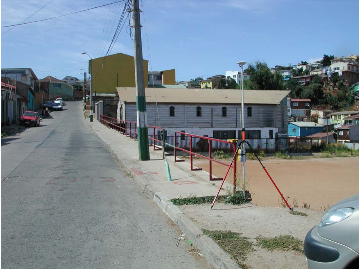
Figure 21: DGPS Rover on site CEMENTERIO.
