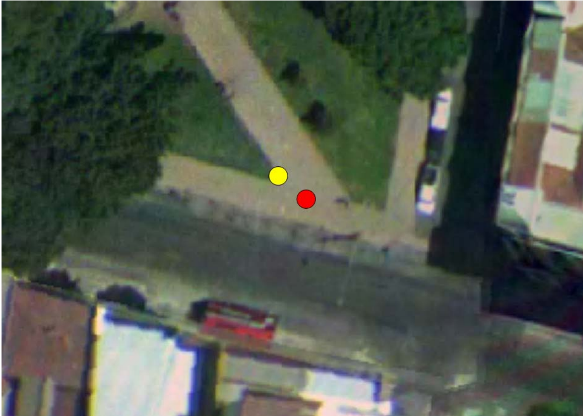
Figure 9: example of shift between aerial photo (red) and DGPS measurement (yellow).
