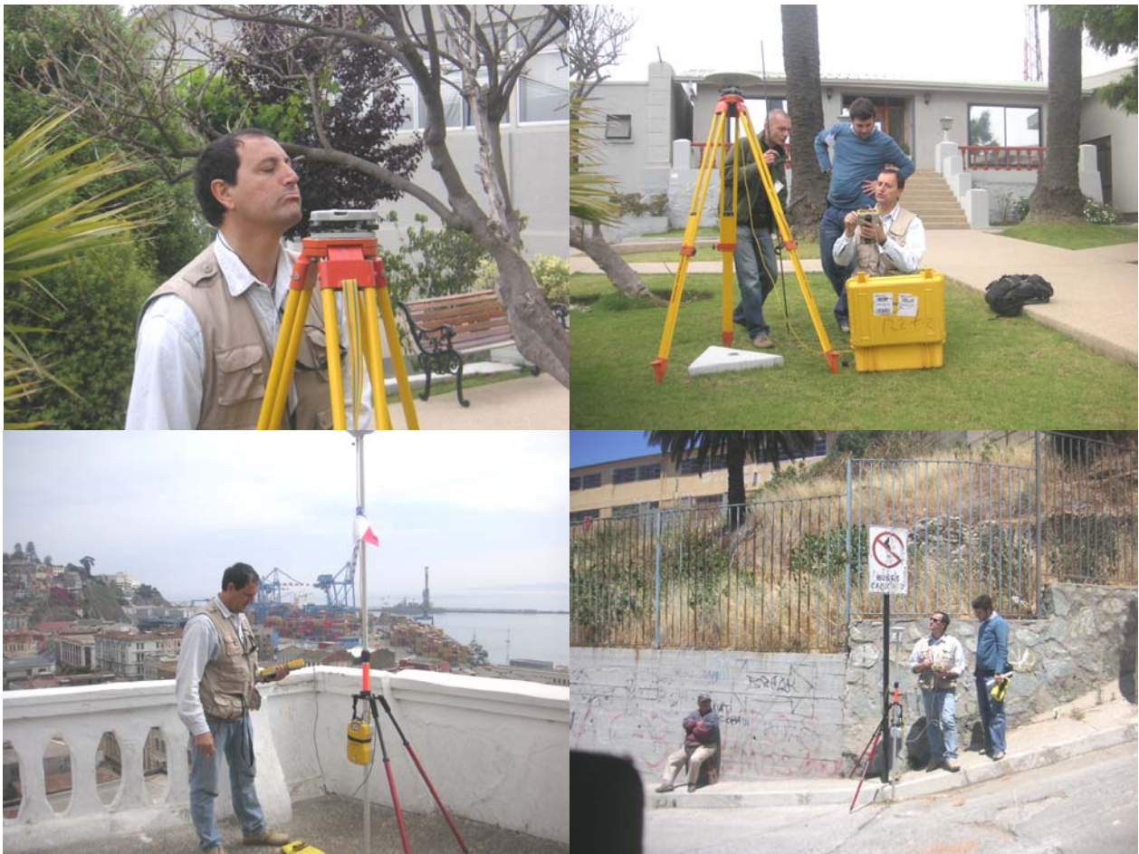
Figure 4: the in field DGPS survey.
