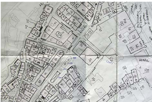
Figure 42: The diagram used for the in field survey, recording the adjustments with respect to buildings, internal building partitions, demolitions, etc.
